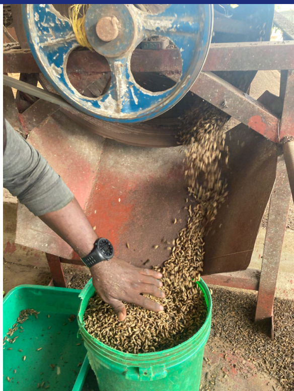
Separating BSF larvae from frass Credits: Photo taken at Chanzi BSF farm in Dar es Salaam, Tanzania
